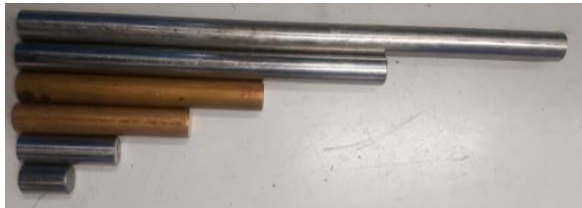
Figure 9. Cylindrical projectiles with masses 250g, 500g, 1000g, 1500g, 2000g, 3000g (bottom to top).
